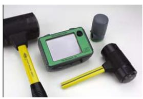
The Low Strain Dynamic Pile Integrity Test has been used for a long time as a method to test the integrity and length of foundation piles.
